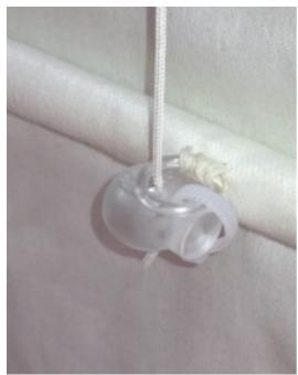
You must ensure that the cord connector for up to four cords is the breakaway cord connector supplied. After four cords a normal cord connector may be used but the cord connector must be installed at a maximum 50mm from the headrail when the blind is in the fully extended position.
